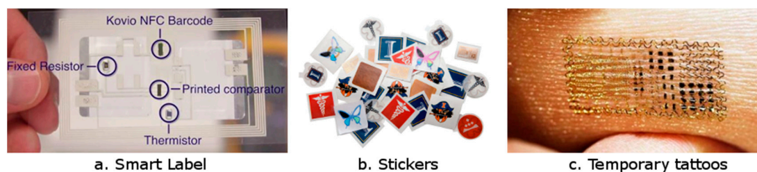
Figure 5. Comparison of micro-thin sensors. (a) Smart Label composition (b) Sensors embedded in stickers; (c) Sensor directly printed on the skin [76,78,84].
