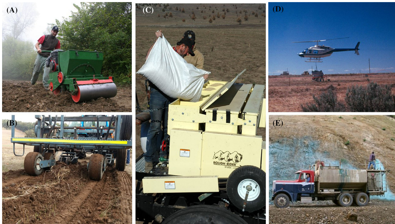
Figure 4 Seeding equipment: (A) Motorized seed mix delivery broadcaster for small-scale projects. This broadcaster provides some degree of seed-to-soil contact but requires a prepared seed bed (Romagnese, Italy). (B) Custom-made precision seeder for delivery of seed mixes used in reconstruction of farmland to the local reference community in southwestern Australia. (C) Minimum-till drills reduce surface disturbance. The triple seed box provides for separate seeding and even flow of large, small, and fluffy seeds. (D) Helicopters can seed irregular areas in rugged terrain and do not require a landing strip. Seed in the rotary spreader is dropped onto a spinner for distribution, but spread is affected by flight elevation, wind, and seed characteristics. (E) Hydroseeding a road cut in Oregon, U.S.A. Photos: (A) S. Pedrini, (C, E) U.S. Forest Service, (D) H. Wiedemann.
