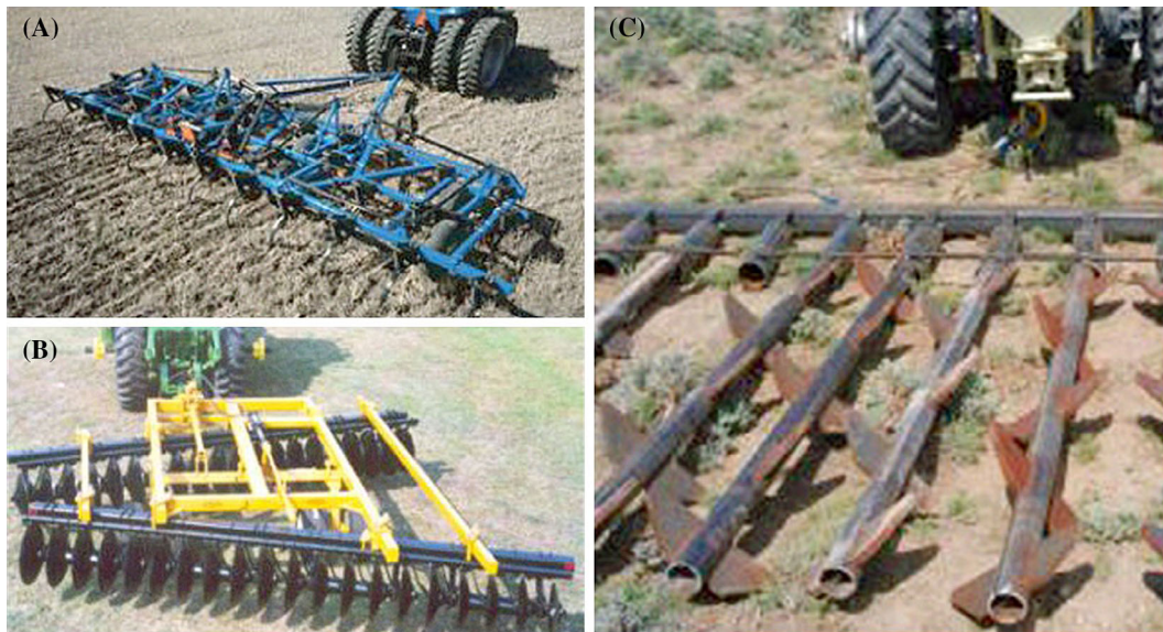
Figure 2 Mechanical seedbed preparation equipment: (A) Chisel plows are used for conservation tillage to control weeds, increase infiltration, and leave residue on the surface. (B) Mid-size offset disks till friable soils, turn under surface debris, break up surface crusts, and uproot shallow-rooted vegetation. (C) Pipe harrows with spiked pipes can be used on level to rocky and rugged terrain to reduce clods but leaves a rough surface. Photos: H. Wiedemann.
