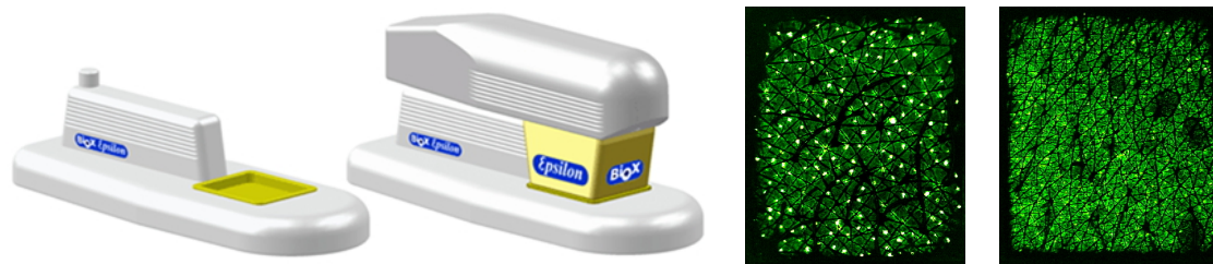
Figure 2. Epsilon™ E100 multi-sensor corneometer (left) and sample scans (right).
