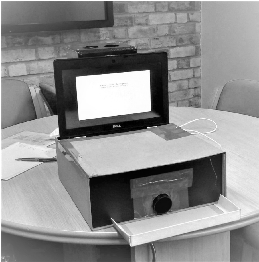
Figure 1. Experimental setup: a touchscreen laptop was encased in a cardboard box. The reward dispenser was placed at the back, and a tube was concealed in the box that delivered encapsulated physical rewards into a small tray at the front of the display.
