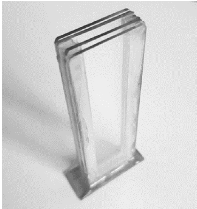
Figure 68 Phononic crystal sensor used for the experimental realizations.
