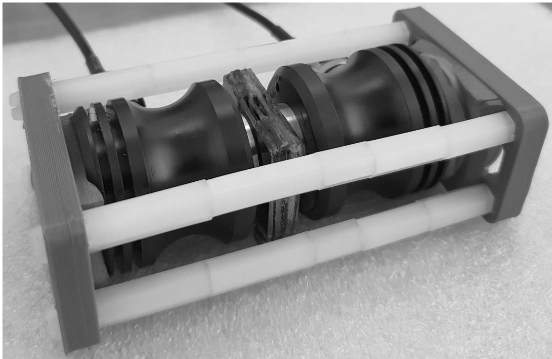
Figure 60 Close up of the experimental setup showing the phononic crystal biosensor, the wideband ultrasonic transducers and a 3D printed support structure used to hold to the setup in position.
