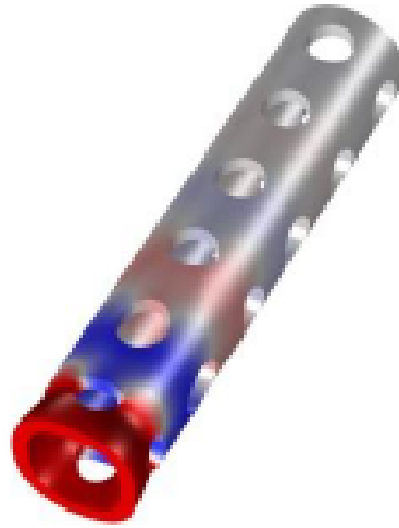
Figure 10 Tubular Phononic crystal structure presented by Lucklum and Pennec. Taken from [112].
