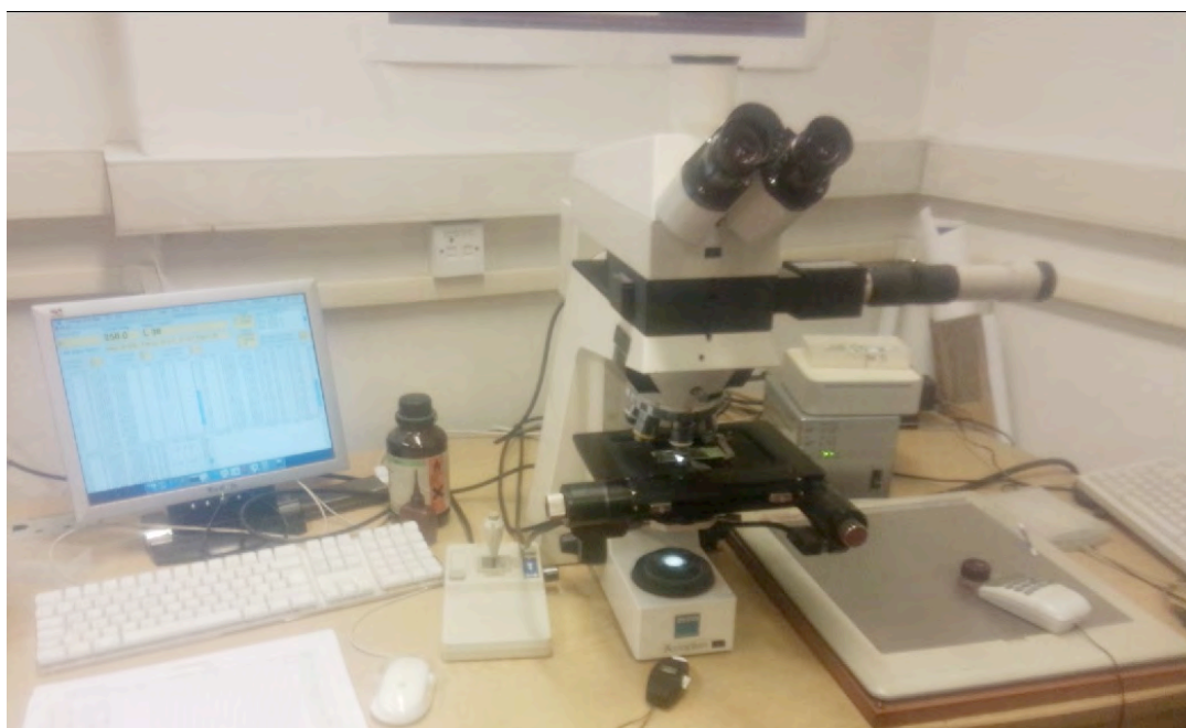
Figure 3.9: The Zeiss Axioplan microscope and stage system used in this study.
