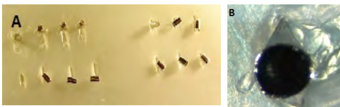
Figure 3.12: A) Rows of platinum tubes pressed into parafilm ready to be loaded with apatite grains. B) close up of a tube which is 0.8 mm in diameter
