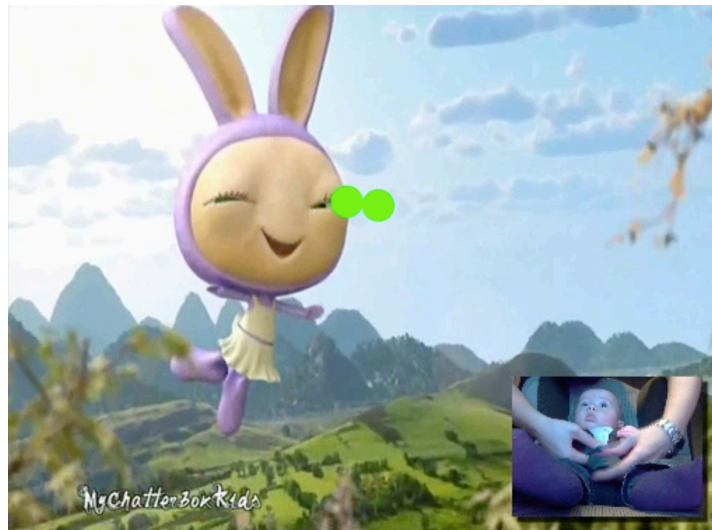
Figure 2-3 Before the calibration procedure starts, the participant's eyes need to be detected. When testing infants a baby-friendly video can be presented on the background while infants are placed in front of the eye-tracker and their eyes are detected.
