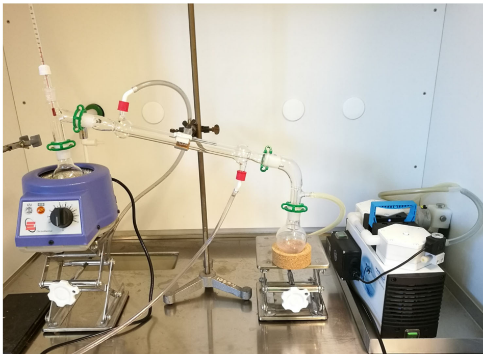
Figure 3: Photo of the glassware of the distillation setup.
