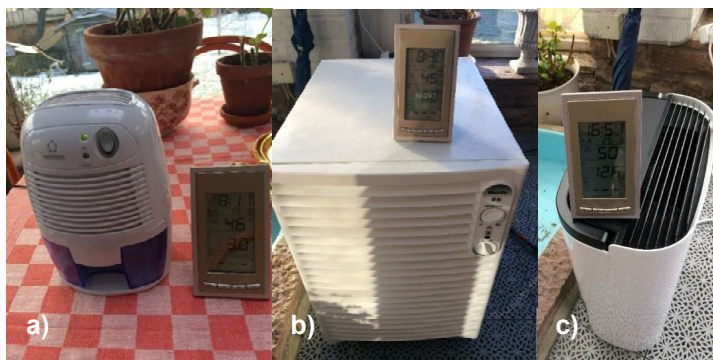
Figure 4: Tested air dehumidifiers a) Renkforce mini; b) Wood's 28; c) Wood's MRD10.
