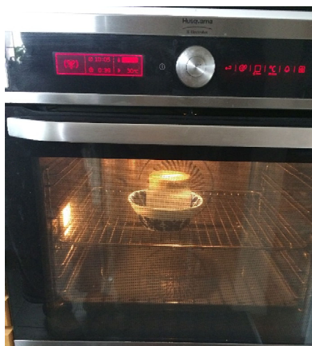
Figure 5: Experimental setup for test of isotope fractionation during evaporation/condensation.
