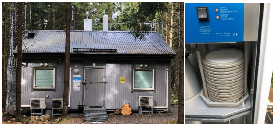
Figure 5: Left: The DHA-80 sampler on the roof of the Hyltemossa site. Right: Interior of the DHA-80 sampler, showing the filters mounted on filter holders.
