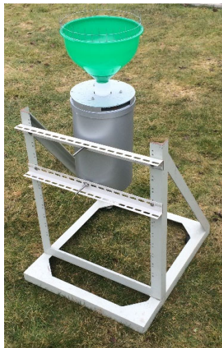
Figure 3: The Palmex rain sampler RS1, equipped with the 23 cm funnel.
