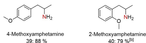
Figure 3. Reductive amination of purely aliphatic ketones and biologically active molecules. [a] Reaction conditions: Fe [10 mol%, 70 mg Fe/(N)SiC with 4.0 wt% Fe loading, 0.05 mmol Fe, 2.8 mg Fe], ketone (0.5 mmol), 140 °C, 20 h, 6.5 MPa H 2 , aq. NH 3 -25% (3.5 mL). Isolated yields of the corresponding hydrochloride salts. [b] 150 °C.
