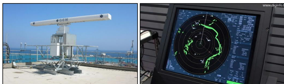
Figure 3 - Marine radar and radar image [10] [11]
