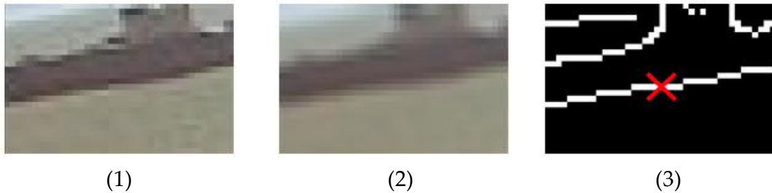
Figure 11 – Removal of the bounding box error. (1) Range of interest (2) Gaussian blur (3) Canny edge detection
