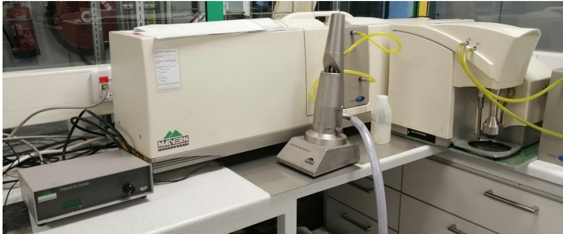
Figure 17. The Malvern Panalytical Mastersizer 2000 laser diffraction testing equipment used for measuring the powder particles size distribution.
