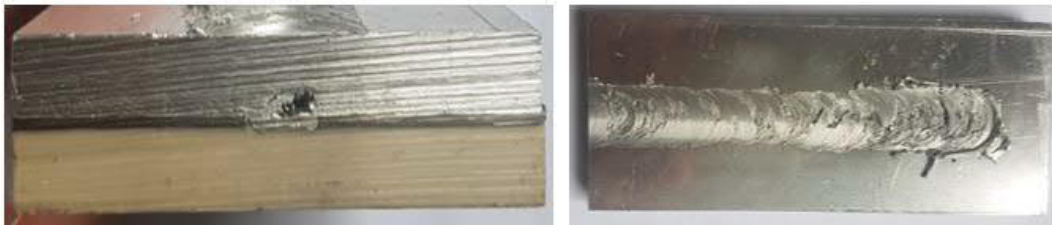
Figure 58: Joint obtained with cylindrical probe and surface features
