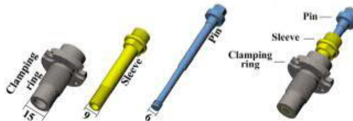
Figure 14: FSpJ tools with principal dimensions in millimetres and final assembly [40]
