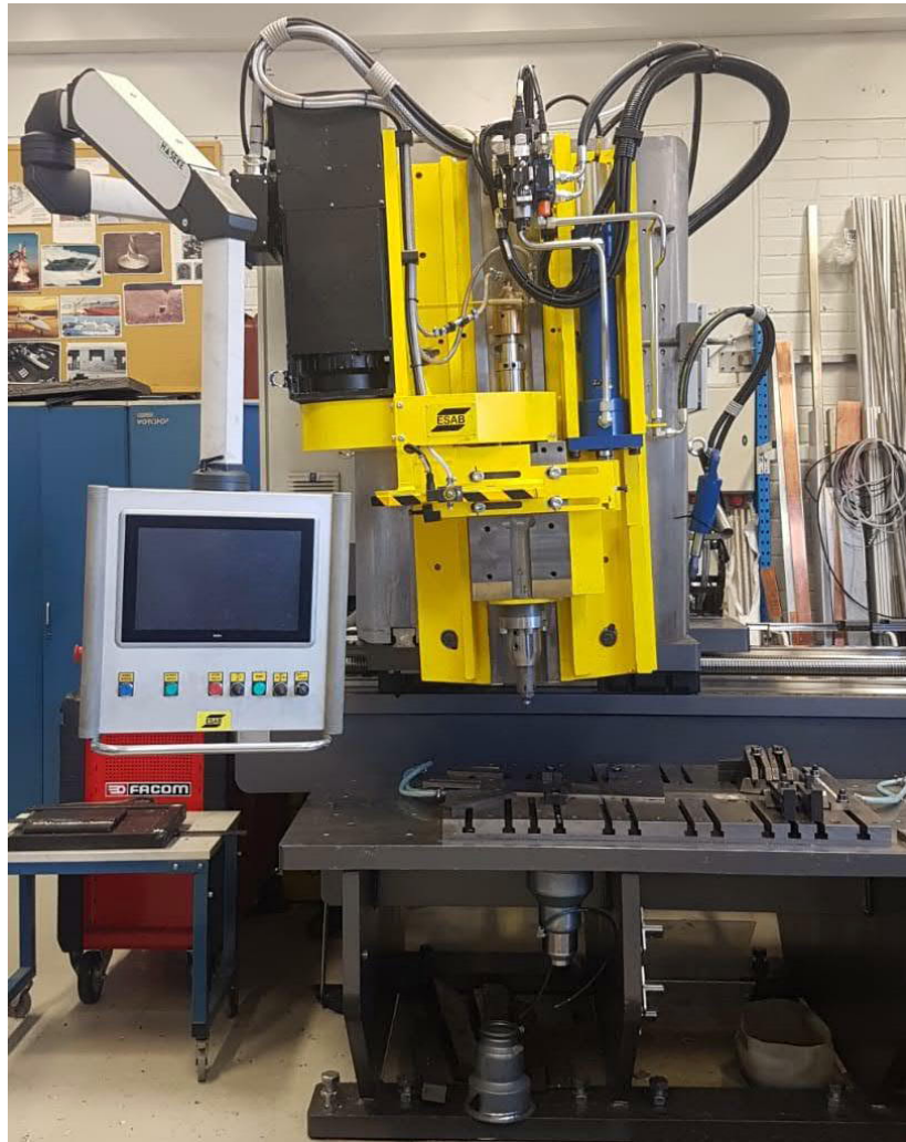
Figure 22: ESAB LEGIO FSW 5 UT available in Aalto University Welding Laboratory
