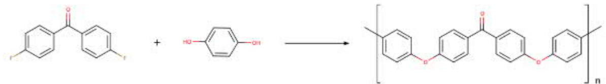
Figure 29: PEEK chemical reaction [64]
