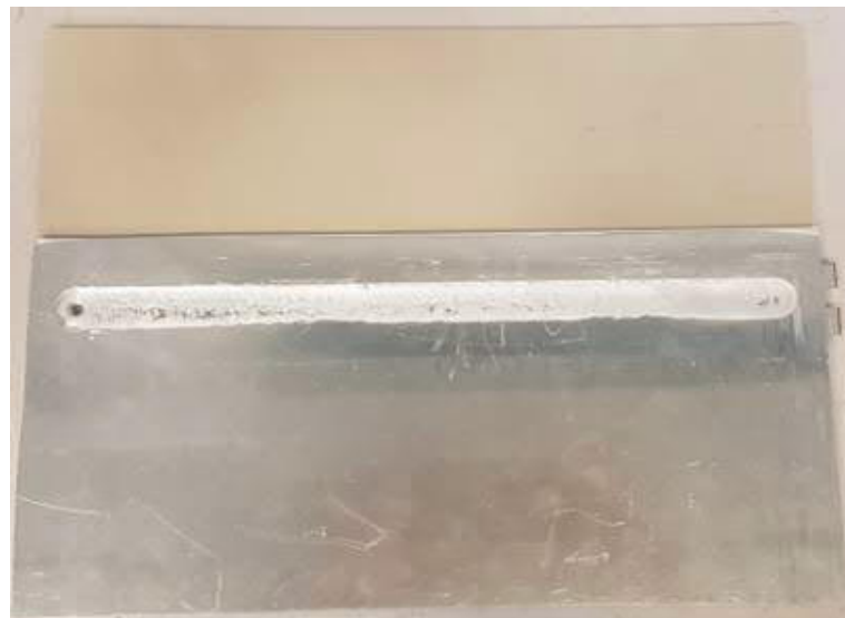
Figure 35: Initial weld test piece
