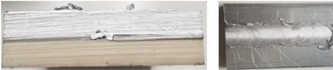
Figure 59: Joint after the increase of the weld depth
