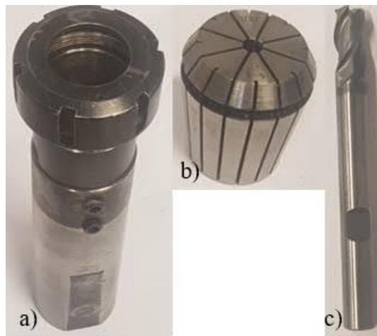
Figure 54: Machining tool, a) collet holder; b) collet; c) mill
