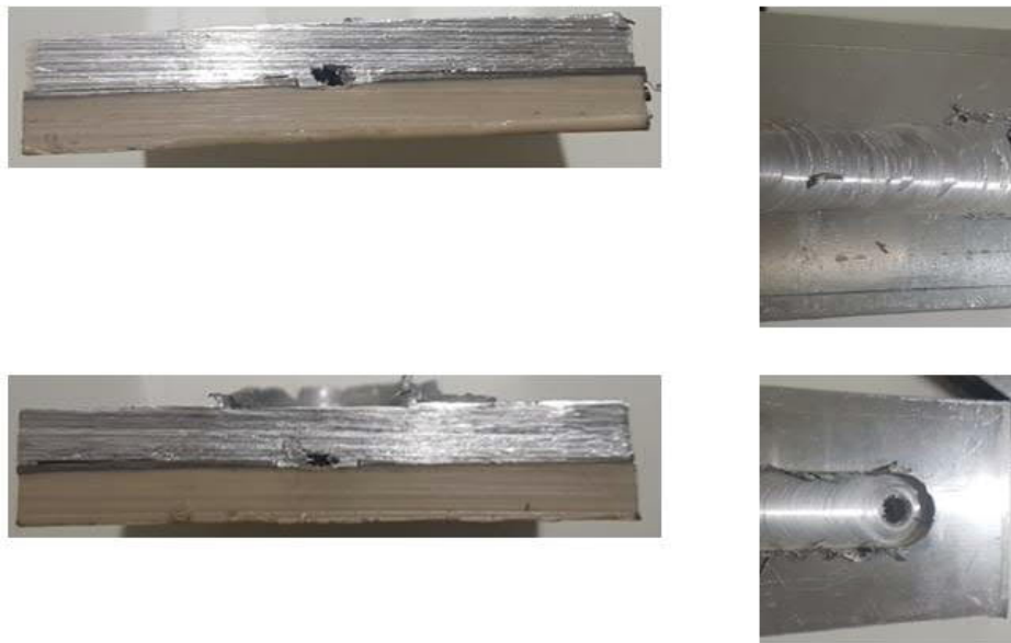
Figure 60: Joint obtained with cylindrical + unthreaded conical probe and surface features
