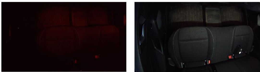
Figure 3.9. Sample images taken with the existing vehicle interior lights (left image) and with the installed LED strip
