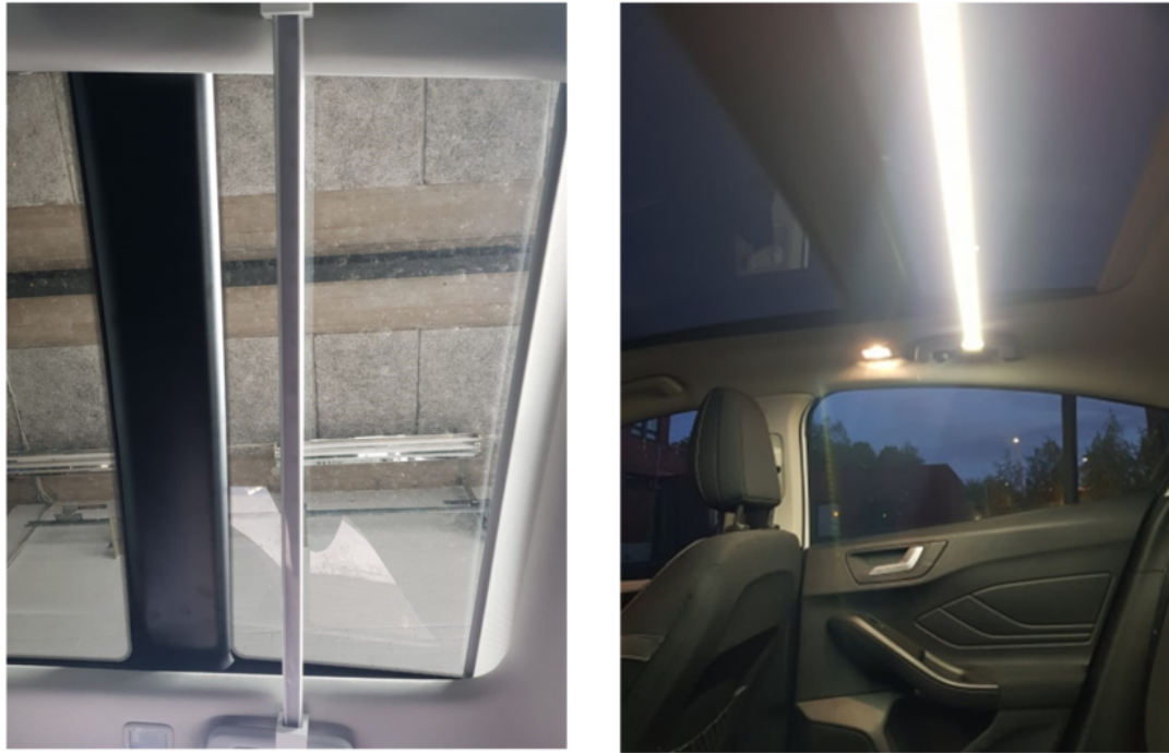
Figure 3.8. Installed light module which traverses over the rear seat in its off and on states
