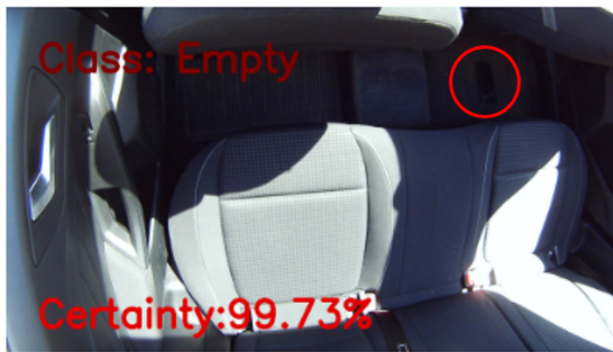
Figure 4.9. A black mobile phone placed on the far end of the floor area is undetected due to its lack of contrast with the neighbouring background. Hence its classified as empty
