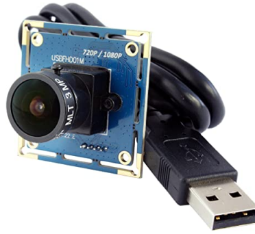
Figure 3.3. USB camera which was installed in the vehicle for capturing the state of the rear seating area (ELP Webcam Wide angle 170 degree Fisheye Lens Camera USB Full HD 1080P 30fps Web Camera for Linux/Windows/android 2015)
