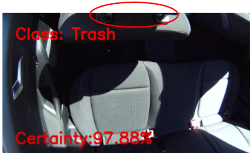
Figure 4.7. An empty seat is classified as trash due to the driver seat being pushed all the way back to its rearmost position
