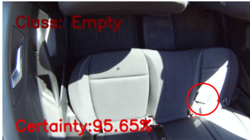
Figure 4.8. A seat containing a mobile phone is classified as empty due to its placement in a bright spot which hinders its detection
