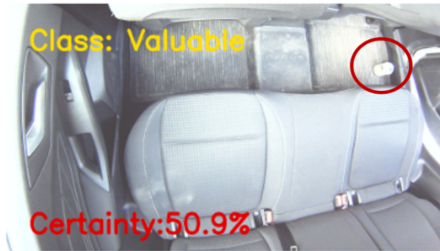
Figure 4.10. A trash can placed on the far end of the rear seating compartment marginally misclassified as a valuable
