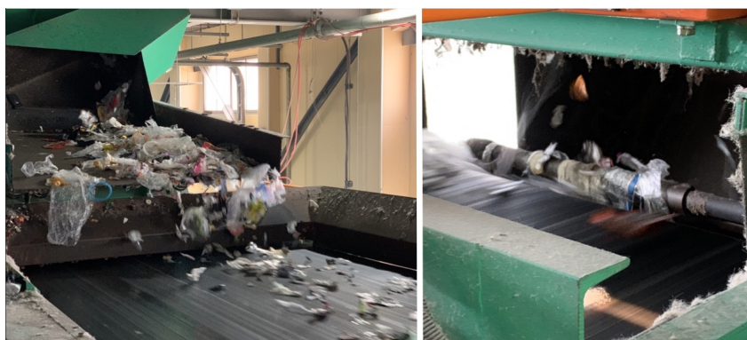
Figure 17: Near Infrared sorting machine at Veolia plant. Upstream (left) and downstream (right) of the sorting process
