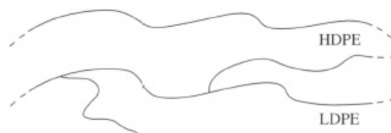
Figure 1: Structures of HDPE and LDPE
