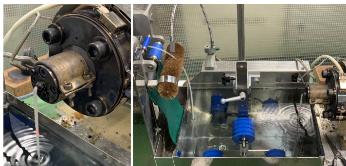
Figure 26: Extruder output (left) and wire cooling bath (right)
