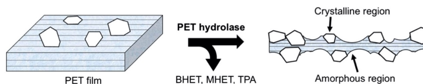
Figure 48: Enzyme degradation occurs preferentially in amorphous zones [200]
