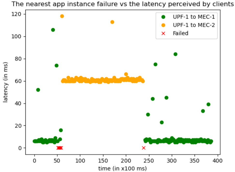
Figure 4.5: The effect of latency perceived by the client when the nearest MEC application instance fails
