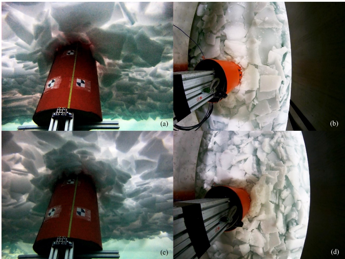
Fig. 5.19 Illustration of rubble size at Test 5 (a & b) and Test 6 (c & d)
