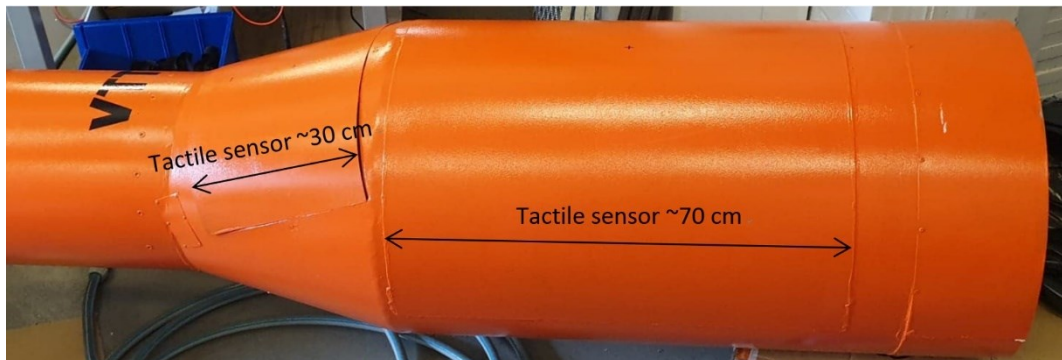
Fig. 3.10 Structure of model, including both cylindrical part and conical part
