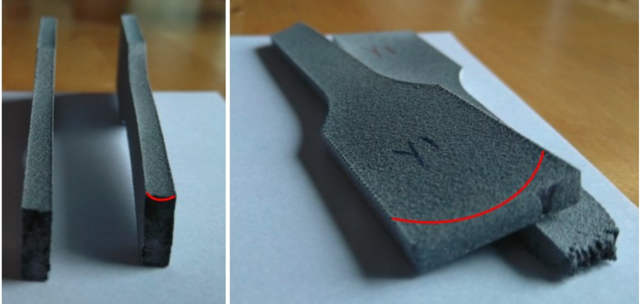
Figure 43: Capillarity present on MJF specimens printed in X (left) and Y (right) directions.
