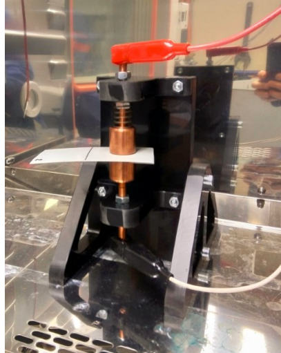
Figure 31: Testing fixture with HIPOT tester cables connected to it and insulation specimen located between the testing electrodes.
