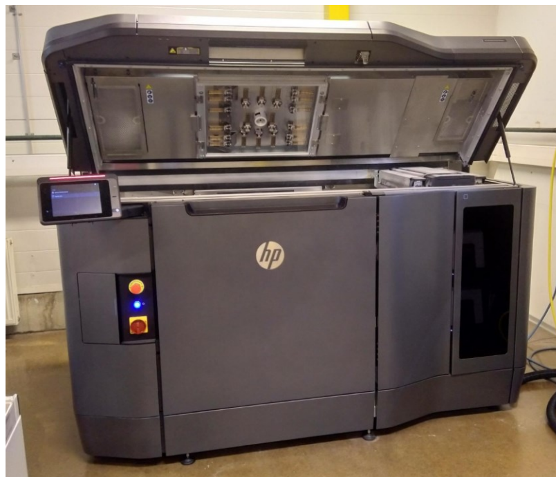
Figure 21: HP MJF4210 3D printing station with upper lid open. Courtesy of Ajatec Prototyping OY.
