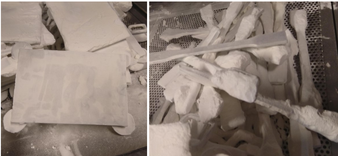
Figure 23: HP MJF parts before cleaning and shot blasting. Courtesy of Ajatec Prototyping OY.
