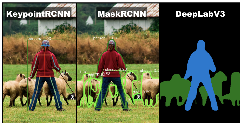
Figure 2.1. Examples of use cases of deep learning with pose estimation, object detection and object segmentation with the respective models KeypointRCNN, MaskRCNN and DeepLabV3. Image from the following blog post - https://pytorch.org/blog/torchvision03/
