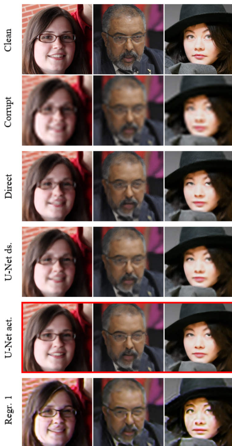
Figure 5.5: Effect of the form of conditioning on the superresolution task. Mean over 5 samples is given for each low-resolution input image (columns). The reference regressive model REGR. 1 (last row) only produces a single answer and hence taking the mean is not useful. The mean results of the U-NET ACTIVATIONS (highlighted with red) model are clearly the sharpest.
