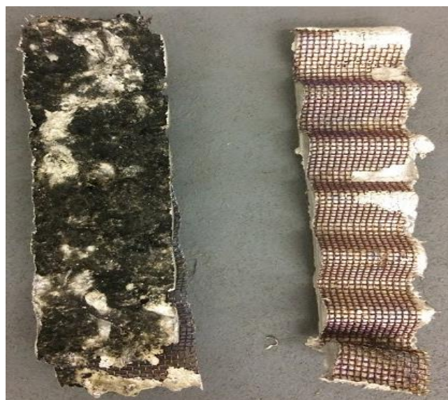
Fig. 2 Stainless steel net over layered with molten and solidified low grade Mg on one side on the net
