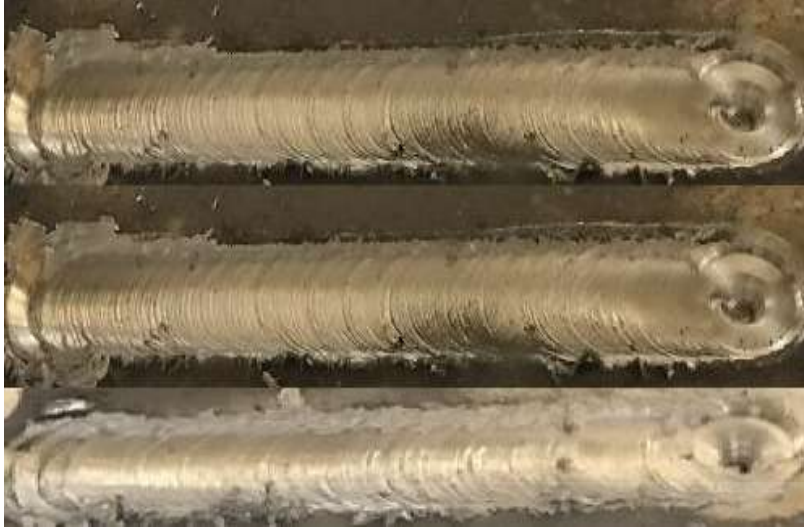
Figure 4. 4 Crown appearance of the processed sample
