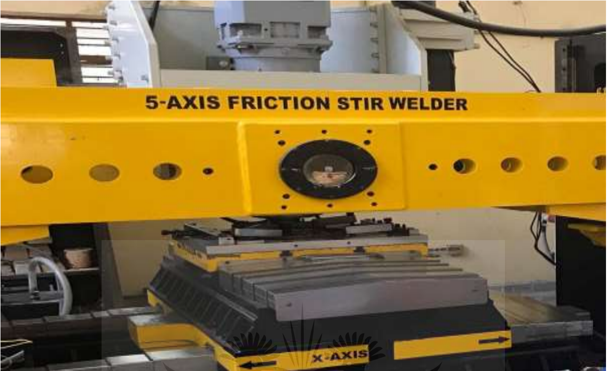
Figure 3. 1 5-Axis friction stir-welding machine used for the friction stir processing of the composites
