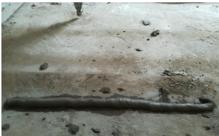
Figure 4.24: Continuous printed strip using final mix
