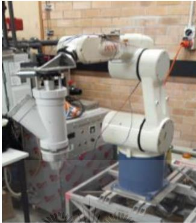
Figure 2.13: 6DOF Industrial Robot
