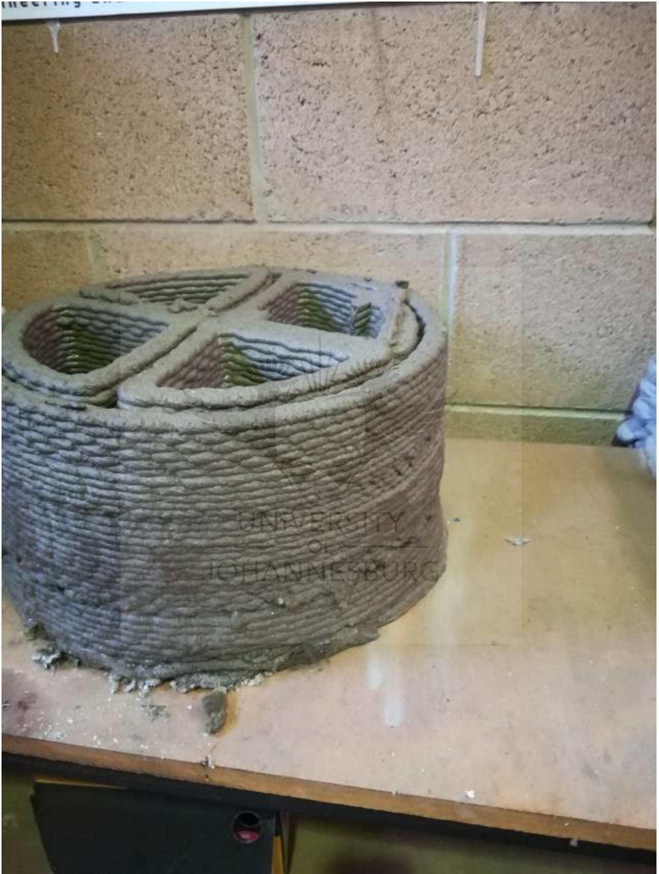
Figure 4.31: Side view of 3D concrete printed structure
