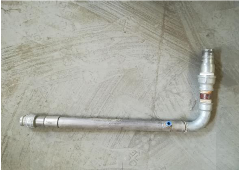
Figure 3.6: Concrete printing head
