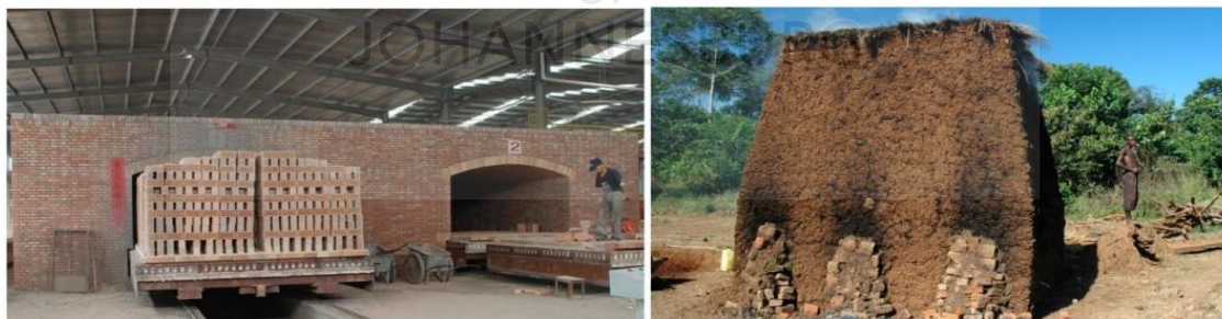
Figure 2.11: Clay brick processing (Left) and brick processing in a rudimentary kiln (right)
