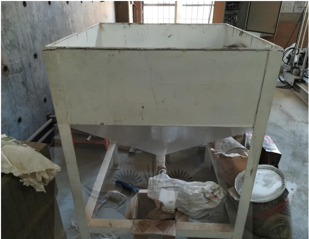
Figure 3.4: Concrete mix reservoir
