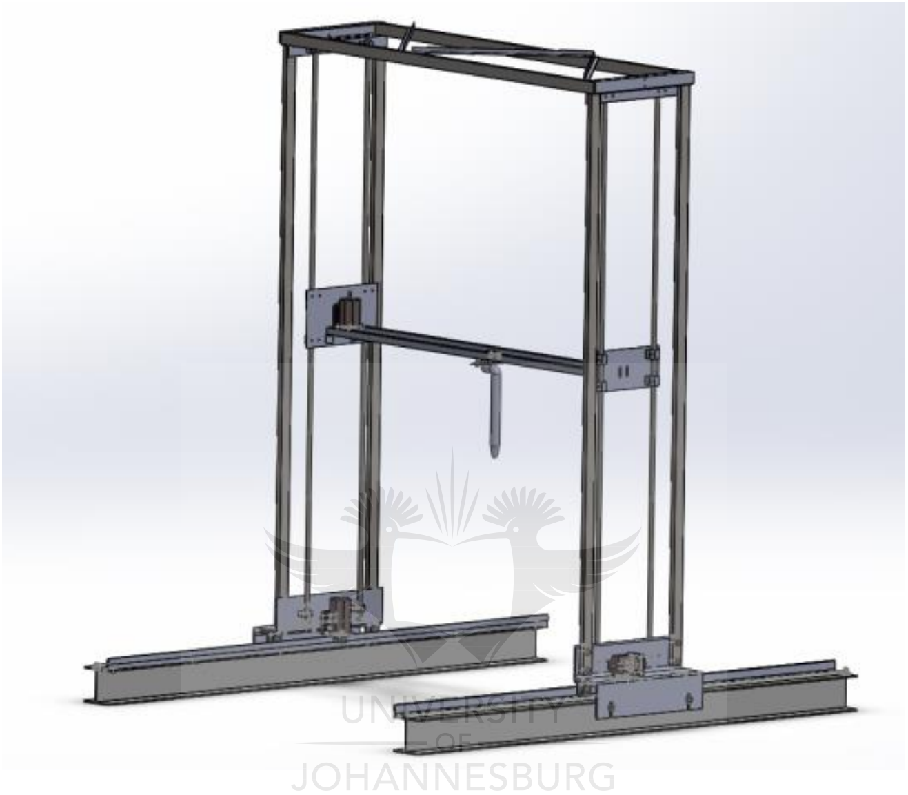
Figure 3.1: Digital design of 3D concrete printing structure
