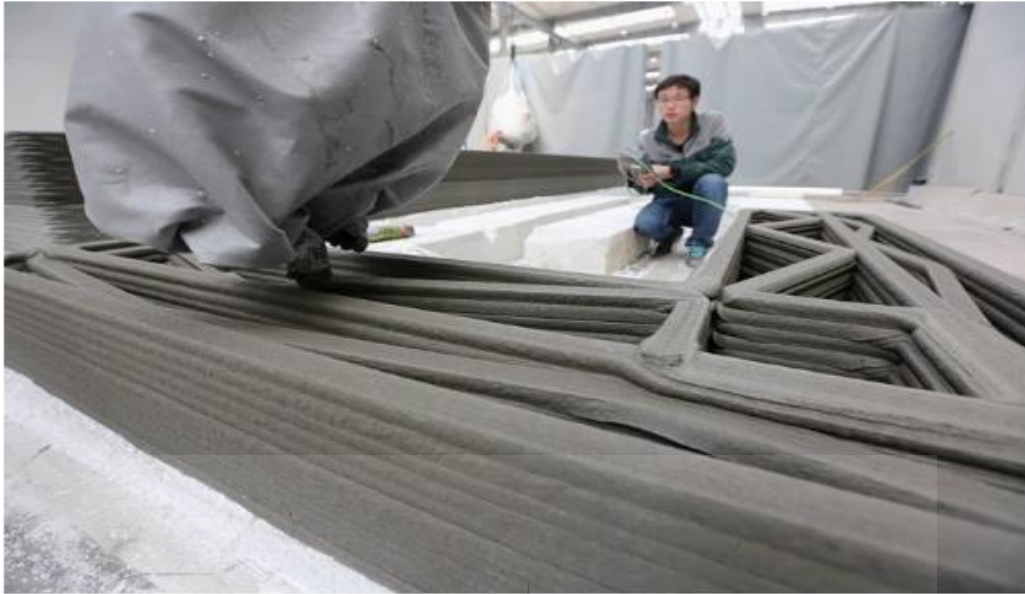
Figure 2.3 Winsun printing concrete (Winsun Decoration Design Engineering Co, 2015).
