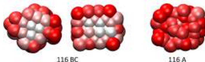
Figure 10. Cuts through 116 NPs showing only Si atoms with the degree of local tetrahedral distortion of the associated [\text{SiO}_4]^{4-} centers indicated by shading (lighter, less distortion; darker, more distortion). Left: two perpendicular cuts through the 116 BC NP. Right: a single cut through the 116 A NP.
