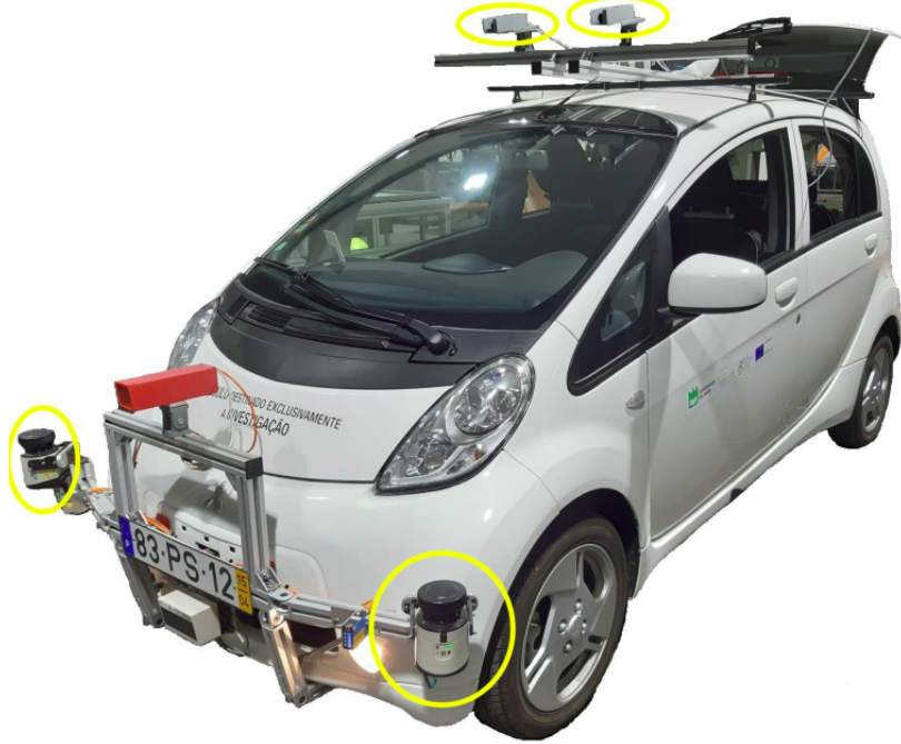
Figure 1.4: ATLASCAR2: Autonomous vehicle from the Department of Mechanical Engineering of the University of Aveiro; the sensors are indicated by the yellow ellipses.
