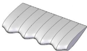
Figure 2.7: Section view of the 0021 NACA airfoil with tubercles [18].
