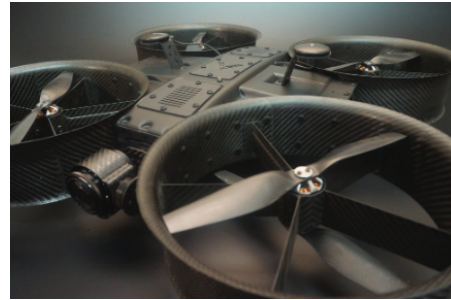
Figure 2.13: Lightweight fan shrouds comprising acoustic materials (Aerotestra MK10) [22].
