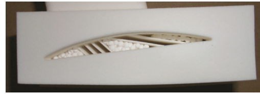
Figure 2.4: Open (no end cap) soft vane configuration; four internal chambers [16].
