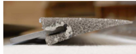
Figure 2.10: Photography of a metal foam trailing edge [20].
