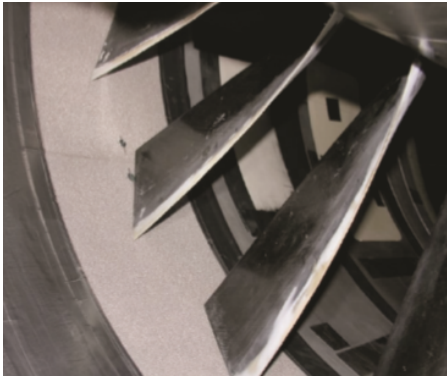
Figure 2.5: Over-the-rotor metal foam liner [15]. [18].
