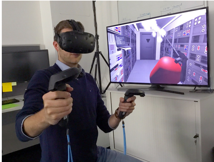
Figure 2.4: Full-immersive VR system with a head-mounted device [ESA 2017].
