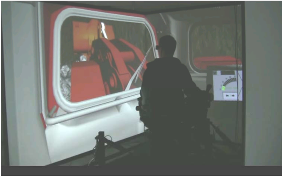
Figure 2.6: Operator testing a virtual prototype in a CAVE system [Kuusisto et al. 2012].
