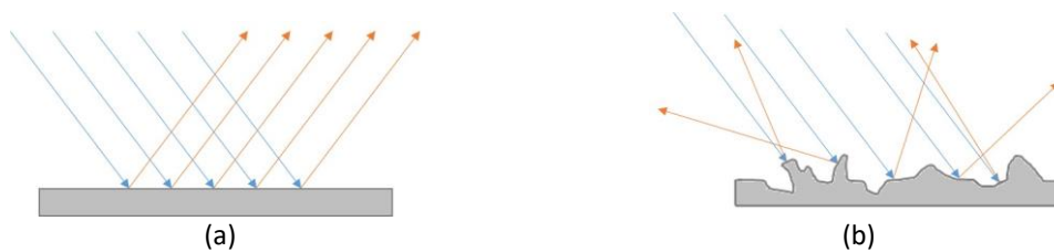
Figure 2.3 Representation of (a) specular reflection and (b) diffuse reflection, after incidence on a smooth flat surface and on a rough and irregular surface, respectively.
