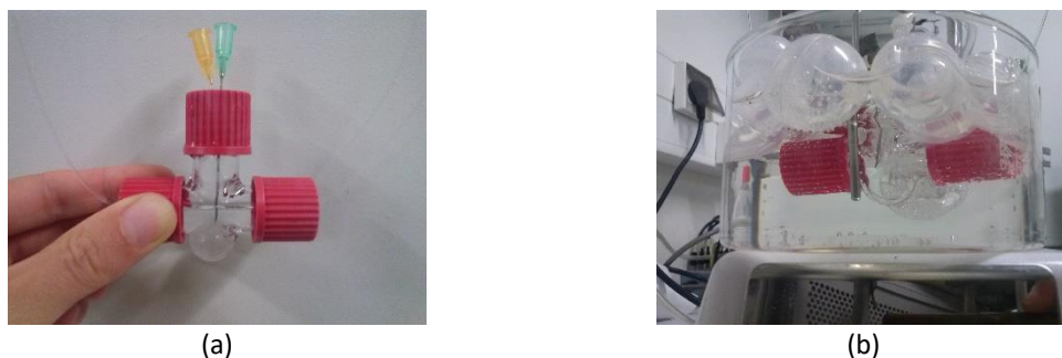
Figure 3.24 (a) Glass reactor with POF and reaction mixture; (b) glass reactor placed inside the thermostated bath for the grafting procedure.
