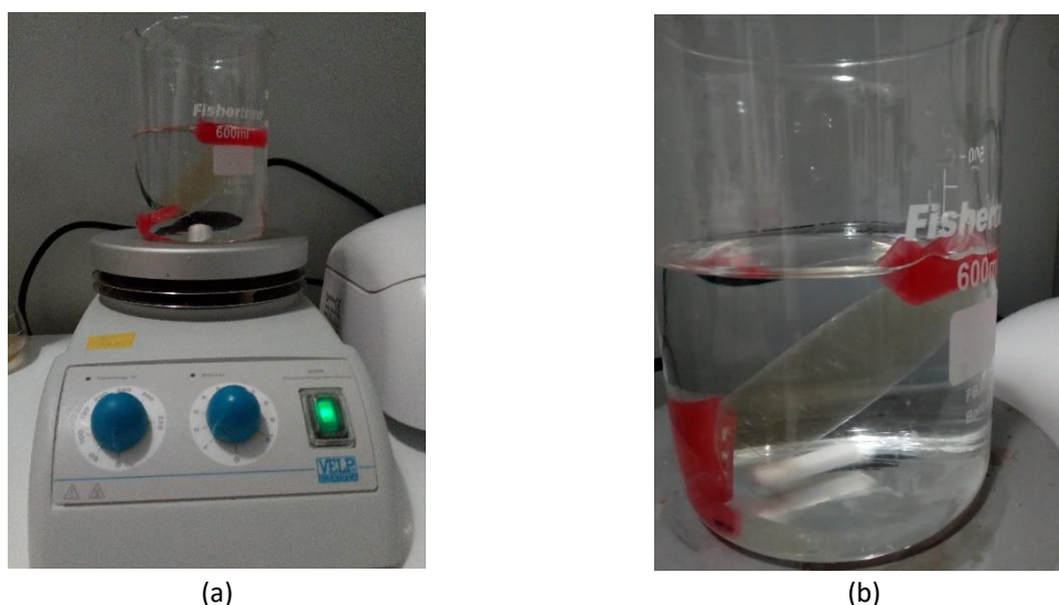
Figure 5.38 Dialysis of the protein solution C: (a) experimental setup; (b) glass vial filled with phosphate buffer and the “snake skin” containing the original protein solution C with Tris buffer.
