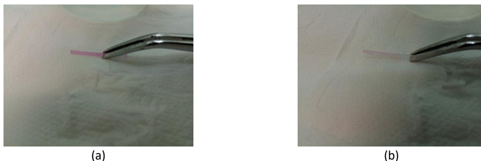
Figure 3.21 Photographs of control sample D2 after: (a) immersion in rhodamine solution overnight and (b) washing with squirts of isopropanol and cleaning with optical paper.
