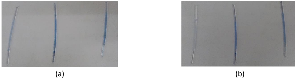
Figure 5.28 POF samples P6, P7 and P8 (from the left to the right) immersed for 1h in buffer and protein solutions, after washing with distilled water (a) and isopropanol (b).
