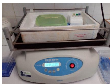
Figure 5.16 Samples of POF immersed in buffer and protein solutions, under stirring (Multi-functional orbital shaker, PSU-20i).
