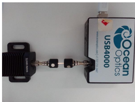
Figure 5.15 Experimental setup: warm White-LED, bare fibre adapters, POF sample and an optical fibre spectrometer.
