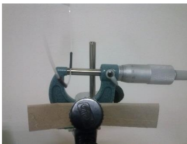
Figure 4.27 Thickness of the sensing region - measurements performed along the length of the sensing region with a Mitutoyo Micrometer.
