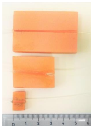
Figure 4.2 D-shaped POF sensors with 1 cm, 3 cm and 5 cm length.
