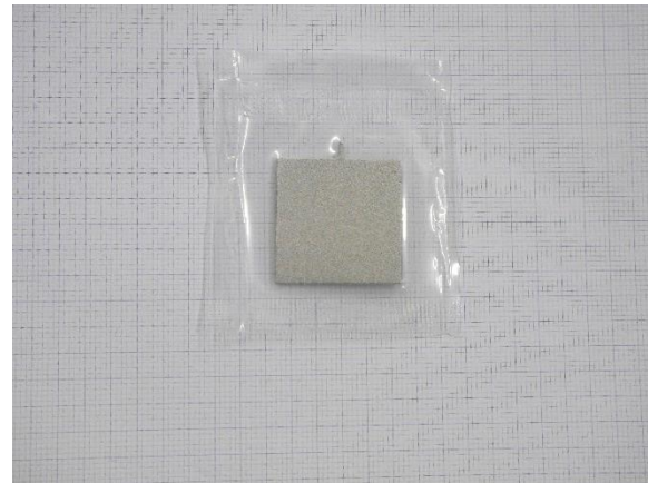
Figure 3.10 Photograph showing the aspect of the PS coatings provided to us by Ceramed. The coatings have an average thickness of 70 \mu\text{m} .
