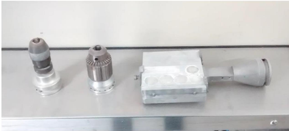
Figure 2.25 Different part tooling available to coat pieces with different geometries. A platform (which is also visible in fig. 2.24) and two mandril tooling are available.
