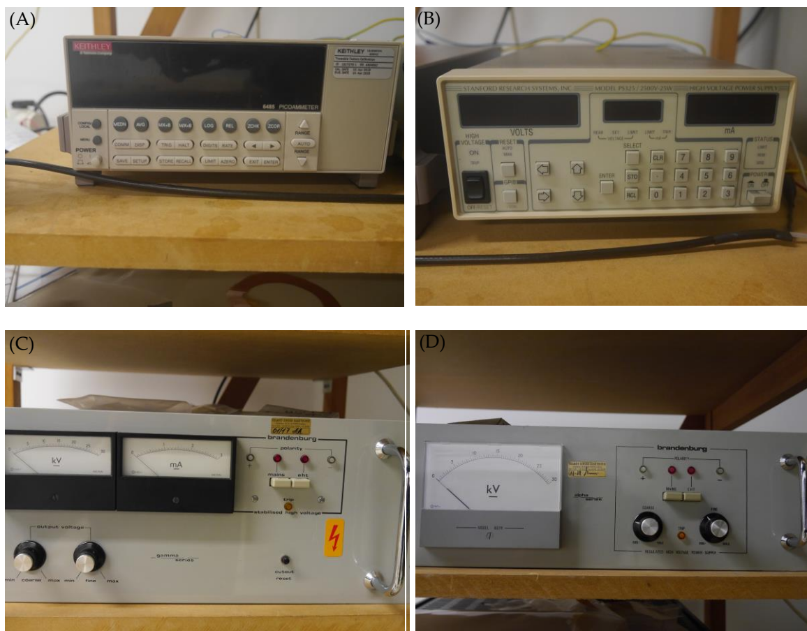
Figure 2.17 The equipment used with the corona triode system. (A) Keithley 6485 picoammeter; (B) Stanford Research Systems, model PS325; (C) Brandenburg model 828-20, from the Gamma series and (D) Brandenburg model 807R, from the Alpha series.
