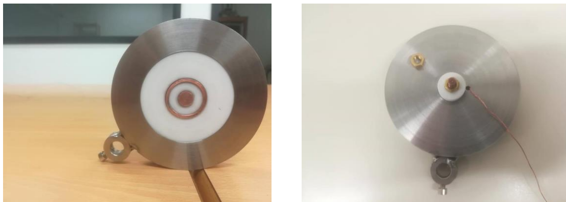
Figure 2.16 Photographs showing top and down perspectives of the metallic support plate containing the teflon support plate for the measurement electrode and the sample.
