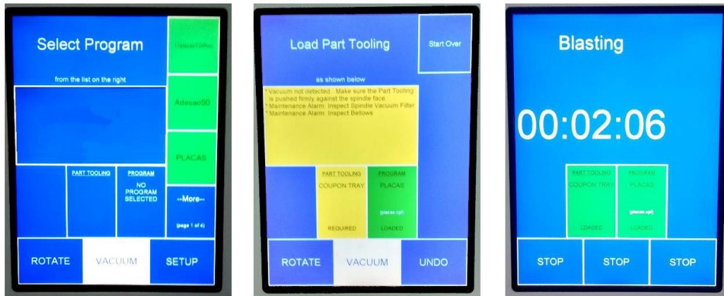
Figure 2.26 The CoBlast system user interface. This interface allows the user to select the coating program, to load the part tooling, to display error messages, etc.
