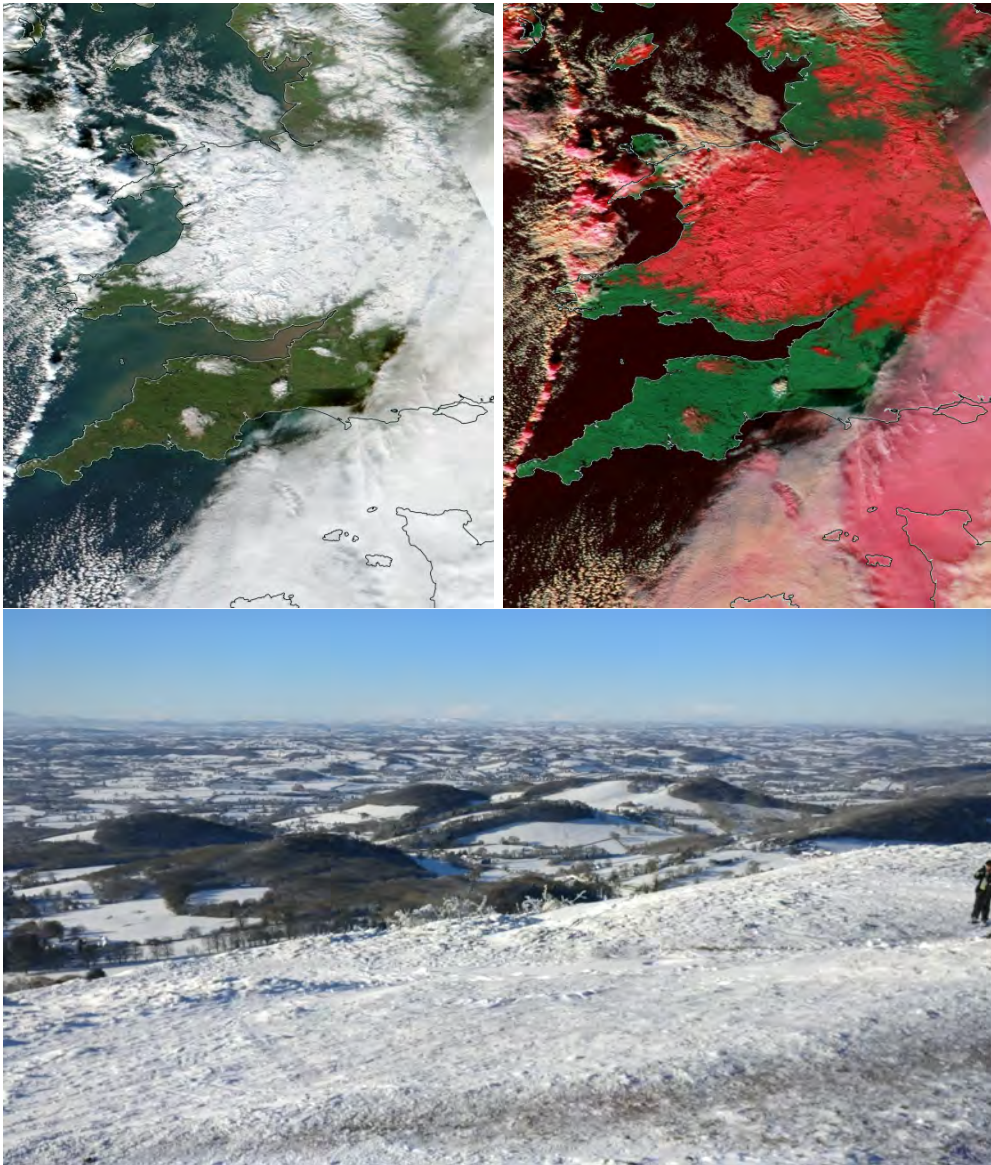
Figure 1 Example images from Suomi-NPP/VIIRS for December 11, 2017, one day after heavy snowfall in large parts of the UK. On the top left true colour corrected reflectance, on the top right corrected reflectance for bands M3-I3-M11 (490-1610-2250 nm). Snow and clouds appear white on the left, but on the right the snow is bright red, clouds either white or pink. On the bottom, a view towards west from the top of The Beacon in Malvern, UK, which is located in the middle of the snow-covered area seen on the top. Suomi-NPP/VIIRS images by NASA Worldview. Photo: Niilo Siljamo (NS).
