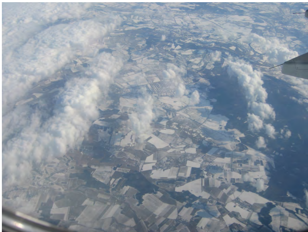
Figure 5 Aerial view of the snow-covered landscape in Germany in March 2006. The photo shows the highly variable and almost chaotic nature of the snow-covered view seen from satellites. Many features complicating the snow detection are present, such as clouds, shadows, variable vegetation and forests. Photo: NS.
