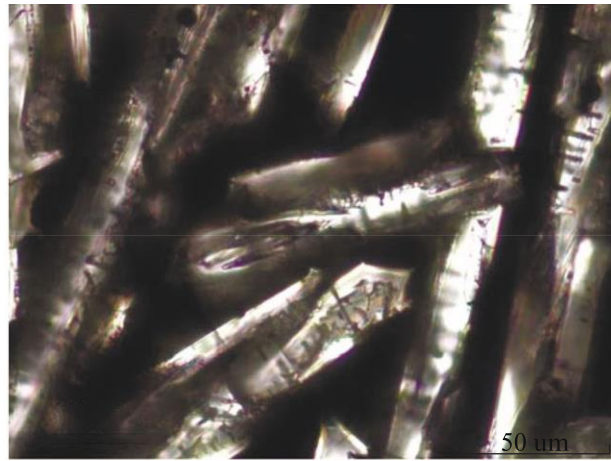
Fig. 3. Optical micrographs of the material produced by experimental shock melting the light-colored lithology of the Chelyabinsk ordinary chondrite: in reflected (left) and transmitted (right) light.
