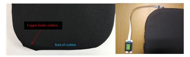
Figure 3. Data Logger Inside Cushion (Left) and Attached to Mat (Right)
