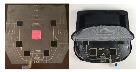
Figure 1. Tekscan Mat Equipped with Force Sensors
