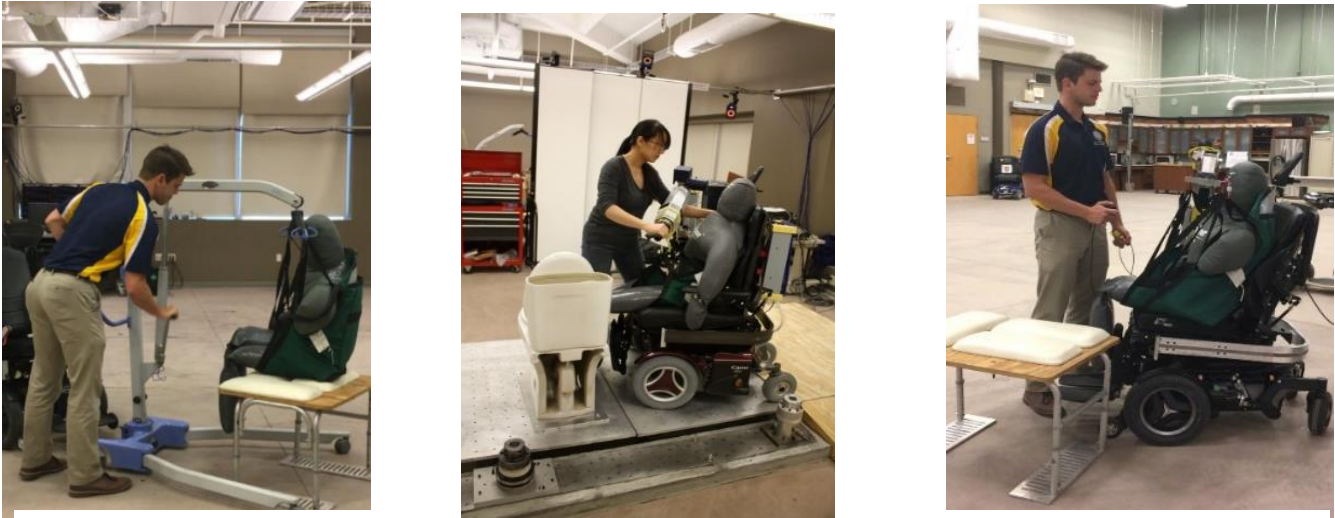
Figure 4 Mechanical floor lift transfer using a lever and compression pump (Top), the prototype of Strong Arm (Middle) and the Strong Arm 2.0 transfer using a joystick (Bottom)
