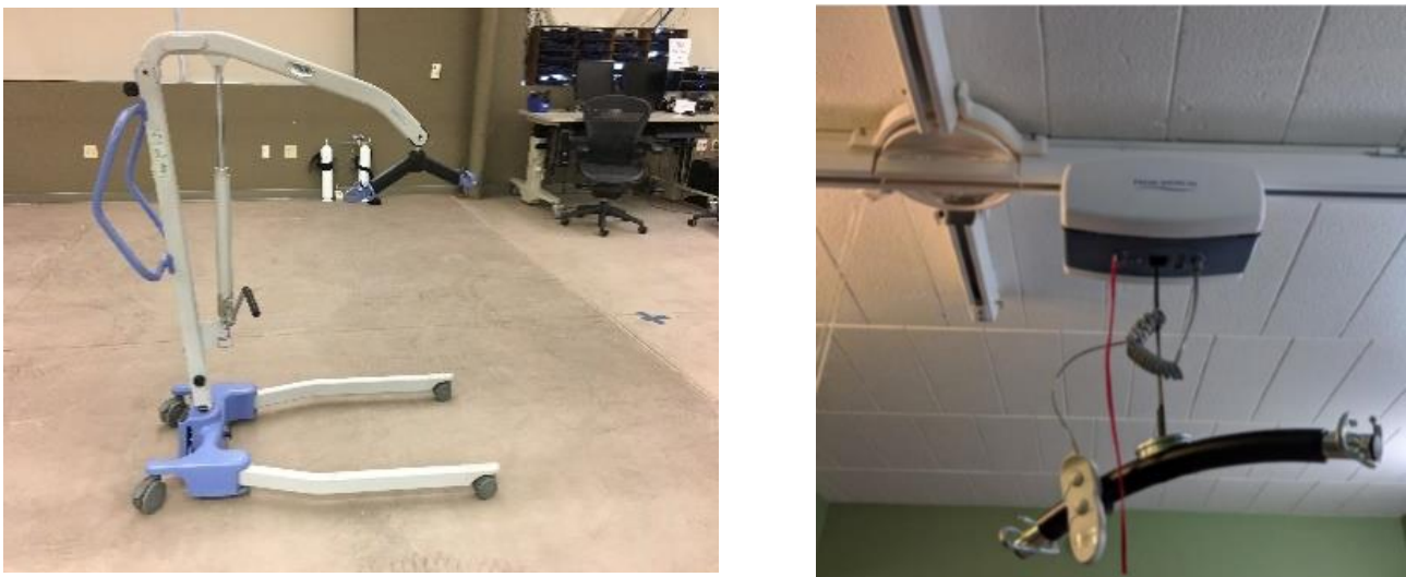
Figure 1 Example of a Floor Lift with a Mechanical Operating System and a Ceiling Lift with an Electronic Based System [33]
