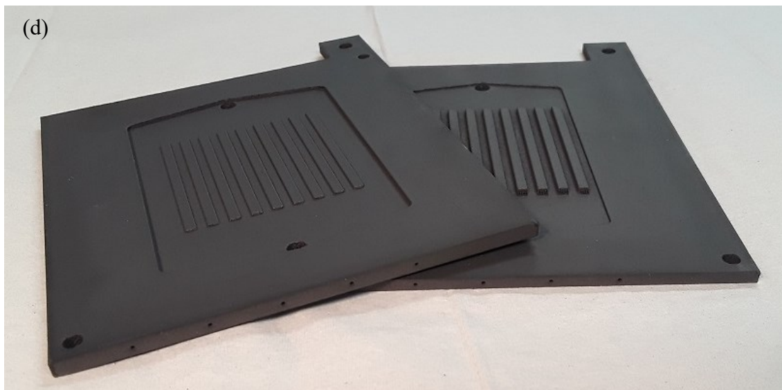
Figure 36 Design schematics with top, side and isometric views of the additively manufacture current-collector (a) anode, and (b) cathode plates. (c) A photograph of the 3D printed current-collector plates. Microstructured channels were carefully implemented during the AM process of electrode fabrication to allow for placement of the distributed fiber sensors apart from the paths of the hot reacting gases. (d) A photograph of the current-collector plates after uniform plating with ceramic, to prevent Cr leakage and prolonging the life-time of the current-collectors.
