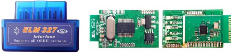
Figure 1: Interface scanner with ELM327 chip
