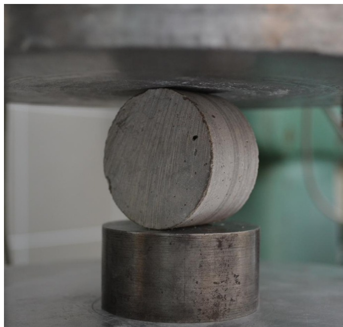
Figure 4: Experimental setup for splitting strength test
