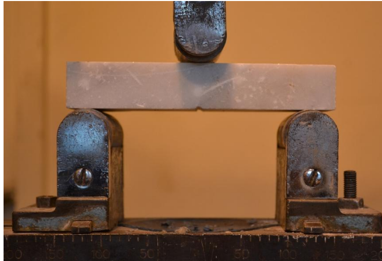
Figure 3: Experimental setup for flexural strength test
