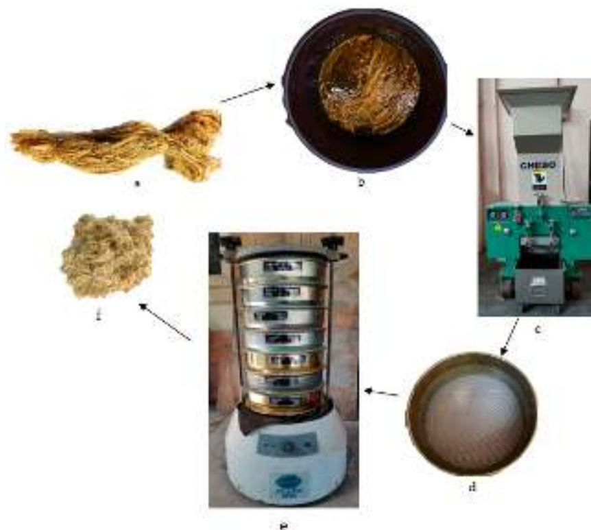
Figure 1. Photos of (a) long banana fibers, (b) chemically retted fibers, (c) fiber chopping machine, (d) 3.35-mm brass frame sieve, (e) rotational shaker, and (f) short banana fibers.
