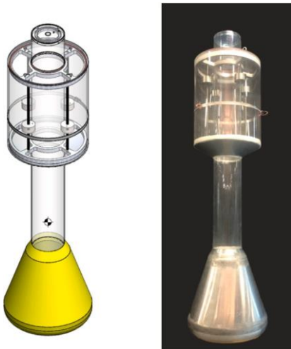
Fig. 11. The spar-buoy OWC CAD and constructed models.
