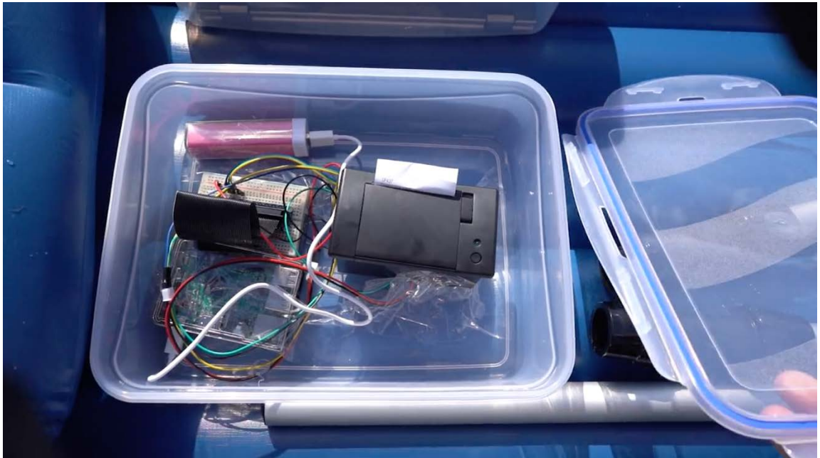
Figure 76: Poseidon's Pull: Revisited (2018) – Raspberry Pi, GPS Tracker and Receipt Printer (by Max Kazemzadeh and Reza Safavi) (Kazemzadeh, 2018, p. 1) - seen above
