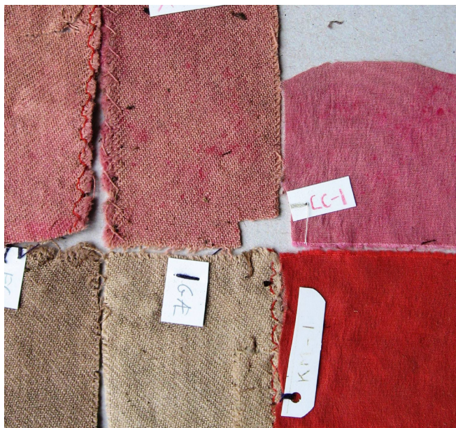
Figure 3 Significant amounts of alizarin and purpurin had migrated from the madder-dyed textile lower left and were found in the cochineal dyed textile centre u. An interpretation of the dye-analysis would have been the textile was dyed clear red with a combination of the two dyes. If the sample for analysis had not been taken in this corner, the results would have been different.
