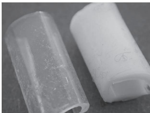
Figure 10.4 Tube before (left) and after thermal ageing at high relative humidity for 65 days. The achieved opacity was reversed on dehydrating under ambient conditions. Sample dimensions: 1.5 mm × 30 mm.
