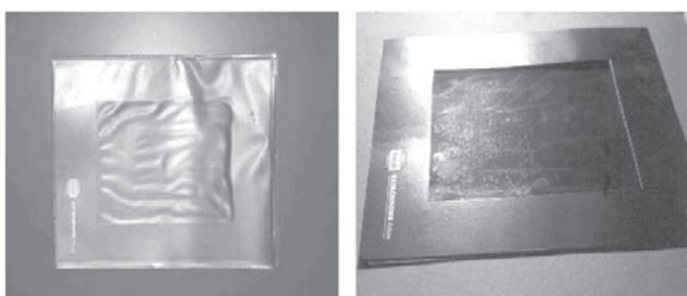
Figure 10.1 Cockled and distorted PVC photograph pocket after 30 years in use (left). Crystalline phthalic acid formed on the surface of the positive image from degradation of DEHP plasticiser deposited by the photograph pocket (right).
