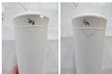
Figure 3. A broken polystyrene cup was adhered with soya and fish adhesives. Soya (left) produced a less visible and more flexible join than fish glue (right)
