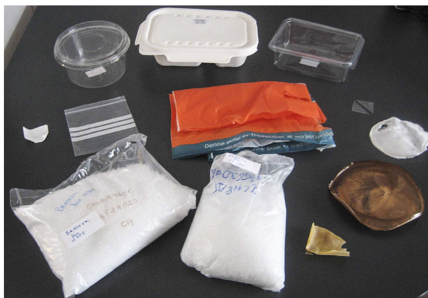
Figure 1. Petroleum-based and bioplastics evaluated: (upper row, left to right) circular PLA food container, fibre box, rectangular PLA food container; (middle row, left to right) Tyvek UV Soft Structure (HDPE), zipper bag (LDPE), PLA/cornstarch bag, Melinex triangles (PET), polyvinyl alcohol film (not examined in this research); (lower row, left to right) bio HDPE, bio LDPE, dried soya adhesive, dried humic acid coating
