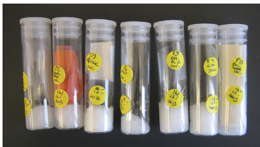
Figure 4. Accelerated thermal ageing of petroleum-based and bioplastics was conducted at high RH and 70°C
