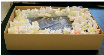
Figure 2. Sample plastics were insulated by loosely packing them with expanded polystyrene chips to slow the rate of cooling
