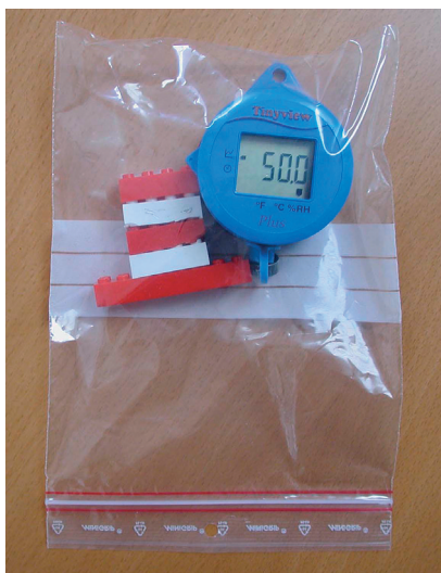
Figure 1. Equilibrium relative humidity of sample plastics was measured by placing them in a closed polyethylene bag with a Tinyview® RH sensor
