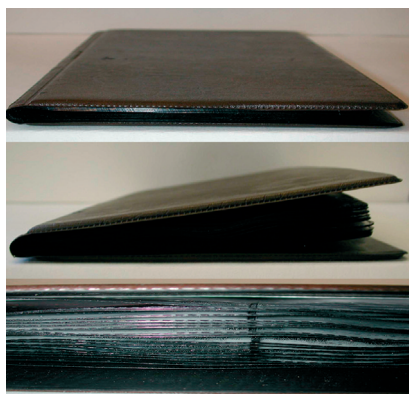
Figure 6. PVC photograph album at 20°C (upper) and at -25°C (middle). Pages of the album were cockled and stiffened on cooling (lower)
