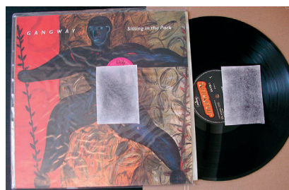
Figure 7. Methylene blue indicator sheets were used to detect the formation of condensation on cooling
