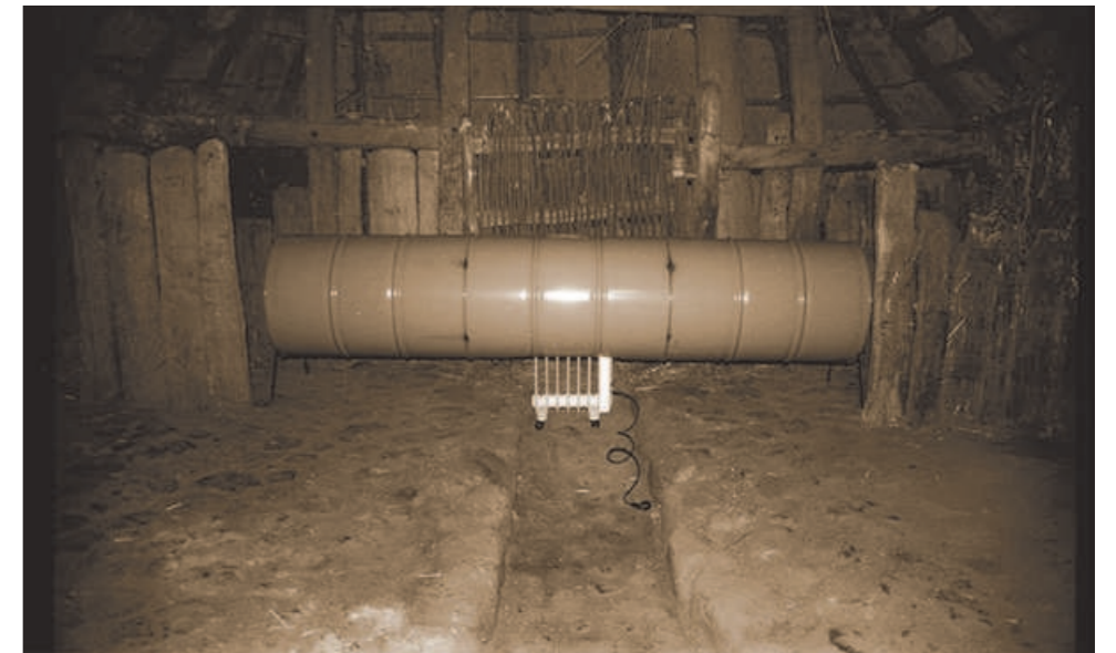
Figure 21 Artificial cows made of oil drums and electric radiators. These “cows” give off as much heat as ten real cows.
