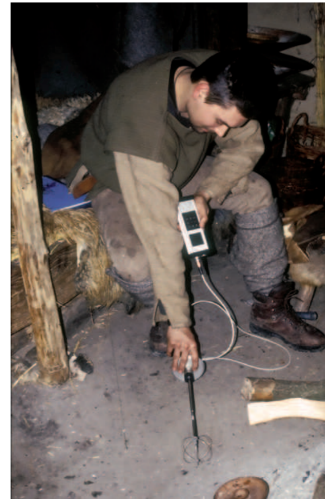
Figure 6 Measurement of draughts at floor level.
