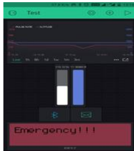
Figure 6. Emergency alarm generated on blynk app
