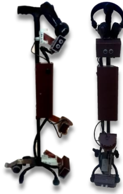
Figure 5. The microcontroller-based guiding stick – front view and right side view
