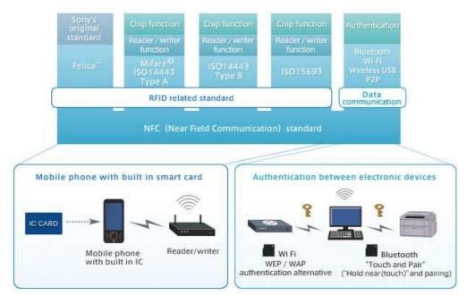
Figure 2. Near field communication standards [2]
