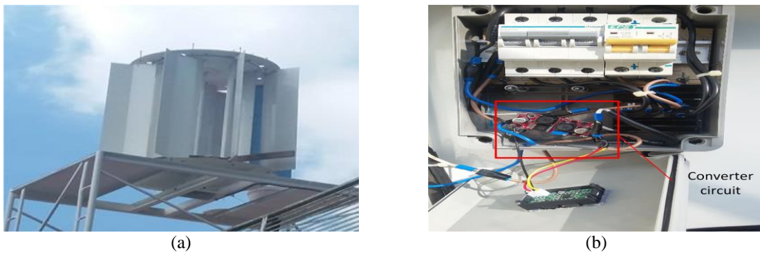
Figure 5. (a) The vertical wind turbine, (b) The converter circuit
