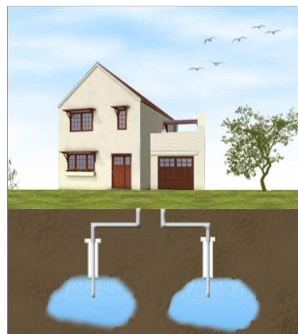
Figure7. Open loop system
