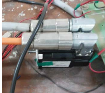
Figure 2. 30 V, 2000 rpm BLDC motor
