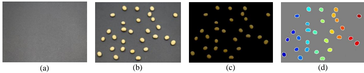
Figure 3. Image segmentation for split soybean seeds: (a) background image, (b) captured image, (c) background subtraction, and (d) region boundaries of each soybean seed
